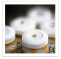
Manufactured at "wafer scale" on silicon, the edible microchips contain copper and magnesium. ~ *Proteus Biomedical*
