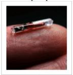
A. An animal microchip implant, also known as a "transponder," is similar to a human microchip implant. (1-2) It is a cylindrical capsule that contains of a radio frequency identification (RFID) device, a tuning capacitor and a copper antenna coil. Although most of the capsules are made of glass, some are made of a polymer material. (3-5)
