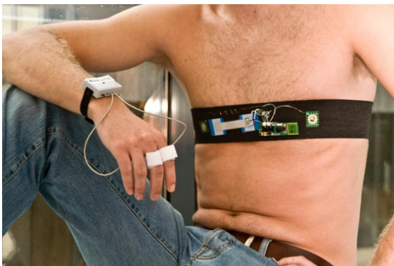
Figure 12. Integrated body area network for ambulatory monitoring of physiological responses from the autonomic nervous system.
