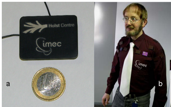
Figure 4. (a) Thermoelectric module for integration in clothing; (b) electrocardiography shirt with integrated thermoelectric generator.
